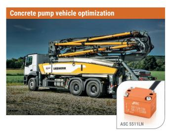
Challenge: Liebherr's innovative, robust truck-mounted concrete pumps are installed on a heavy-duty transport vehicle. Shocks and vibrations are induced in the structure and chassis by the pumping process, as well as by potholes and other obstacles when driving to and from construction sites.
