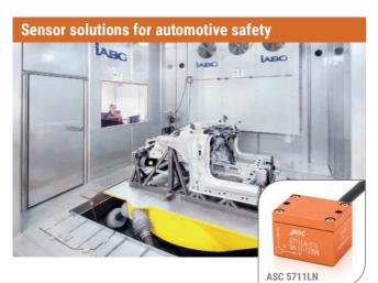
**Challenge:** Truck and other commercial vehicle components can be subject to 90 times the acceleration of gravity in difficult road conditions. Tests are needed to simulate similarly extreme loads up to 2,000 m/s² peak acceleration and over a broad frequency spectrum from nearly 0 to 200 Hz.
